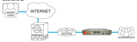
In this scenario, the USC10M2 is placed inside the LAN, in between a router and a workgroup. To access the unit, the admin/user would use the IP address of a member of the workgroup. In this scenario it may be necessary to open specific UDP and TCP/IP ports on the firewall, so that management packets would be allowed through to traverse the IPCopper unit.
