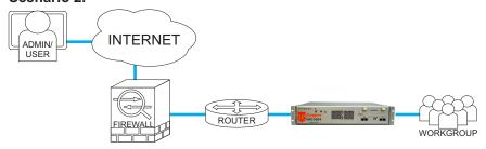
In this scenario, the USC10G4 is placed inside the LAN, in between a router and a workgroup. To access the unit, the admin/user would use the IP address of a member of the workgroup. In this scenario it may be necessary to open specific UDP and TCP/IP ports on the firewall, so that management packets would be allowed through to traverse the IPCopper unit.
