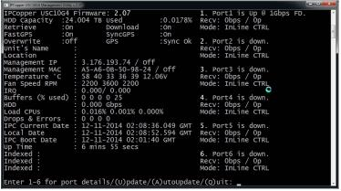
The status page displays the unit's current settings and performance statistics, as well as the status of the individual ports. Entering an individual port number will provide additional port statistics.
