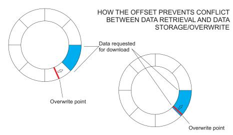
The data retrieval request above encompasses portions of data close to the point at which the oldest data is being overwritten with the newest. During the course of the data download, the overwrite point reached the portion of the data requested for download and the data download failed.
