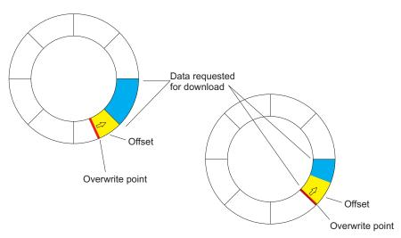
The data retrieval request above encompasses portions of data close to the point at which the oldest data is being overwritten with the newest, however, an offset has been utilized. While processing the data retrieval request, IPCopper determines from which point the requested data starts. If that point is within the immediate overwrite zone, IPCopper will shift the beginning of the retrieval away from the immediate overwrite zone by the specified offset.
