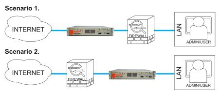
In both scenarios illustrated above IPCopper is located inline on the wire, in one case between the firewall and the internet and in the other case between the firewall and the LAN. In either case, using an IP address from the public internet would cause the management packets to pass through the unit.
