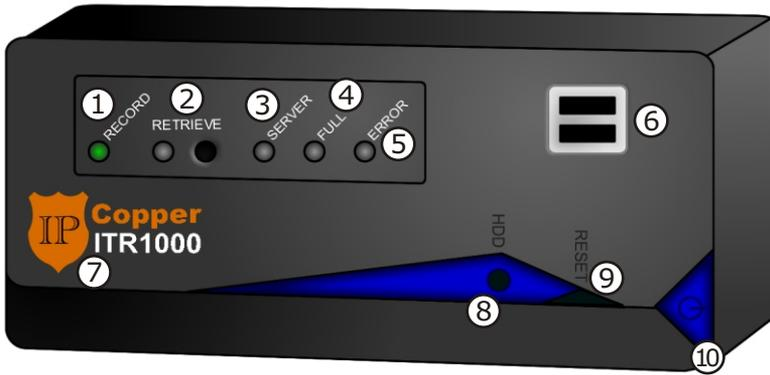
1. Record LED: This light indicates that the unit is recording.
